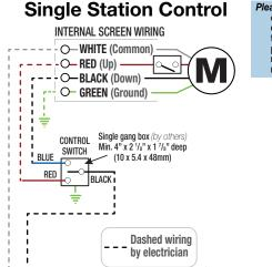
Please Note: Test divider operation. If divider direction does not correspond with the switch orientation, turn power back off and switch the red and black wires from the motor to the switch.
